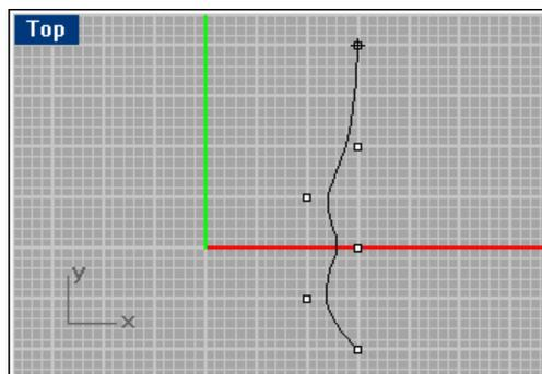
Define the curve with the help of control points (or any other curve command)
