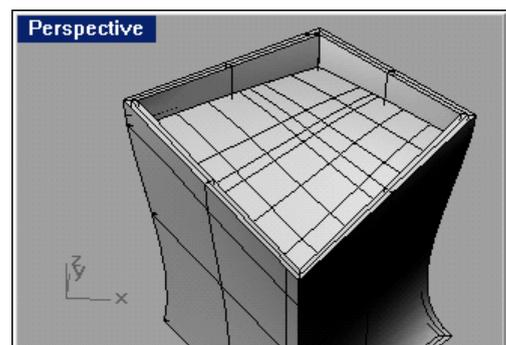
Result from *EdgeSrf* command with second projected curves
