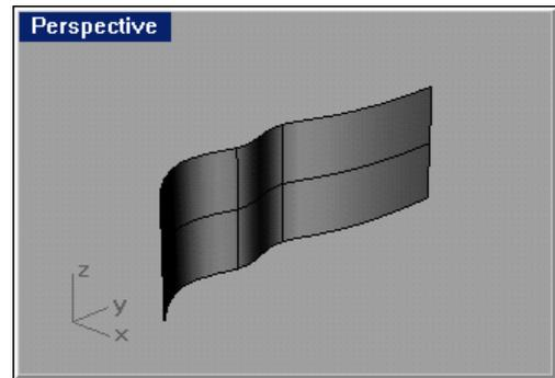
Result of extrusion of a curve into a surface (2)
