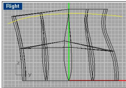
Curve that represents the ceiling cutting the structure – for the outside surface
