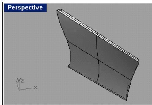
Result of lofting all edges and joining them together – one side of the structure
