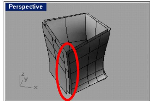
Result of the *OffsetSrfc* command – the outside surface edges don't match. If the offset was done outside to inside then the surfaces would intersect
