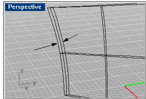
Results after do the lofting in the left border (keep the *Straight Sections* selected in the *Style* and also the *Do not simplify* in the *Simplify* to achieve best results).
