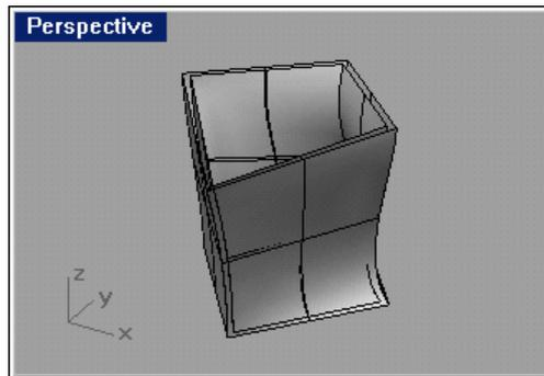
Result of lofting with straight sections – two *PolySurfaces*
