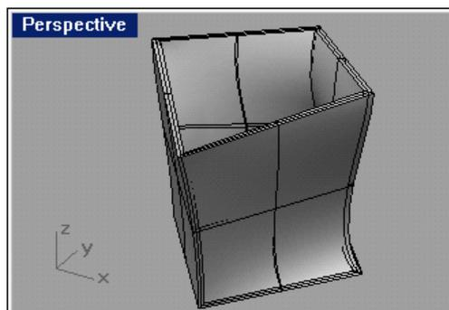
Result after lofting and joining all the walls
