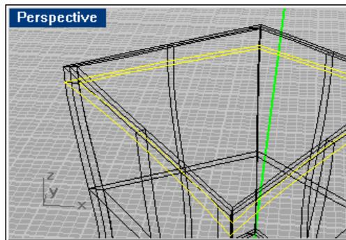
Result from projecting the curve into the structure – the project command was done in the *Right* viewport. As you can see there are 2 curves project for each wall
