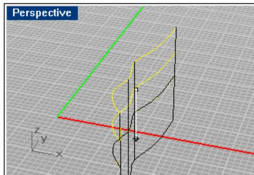
Incorrect extrusion direction
