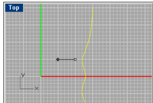
Defining a new vector for extrusion is like draw a line, the endpoints define the line and its direction the direction of extrusion
