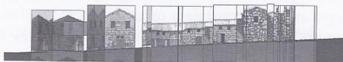
Figure 4. Flank of a street with elevation drawings applied as materials to building blocks.
