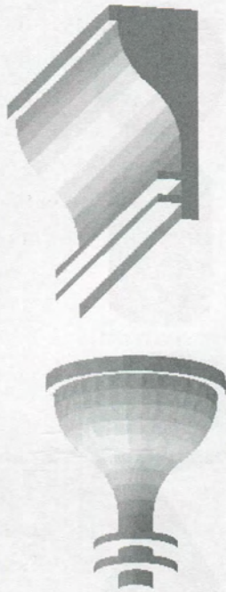
11.15 Solids of translation and revolution produced from the same profile
