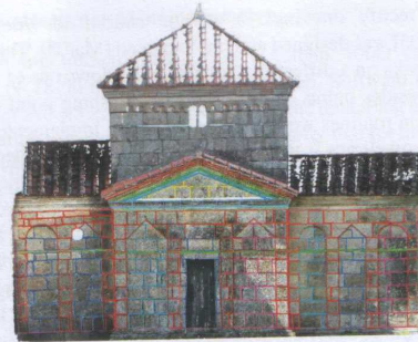
Figure 5: Drawing rectification elevation drawing overlapped to laser scanning ortho-image.
